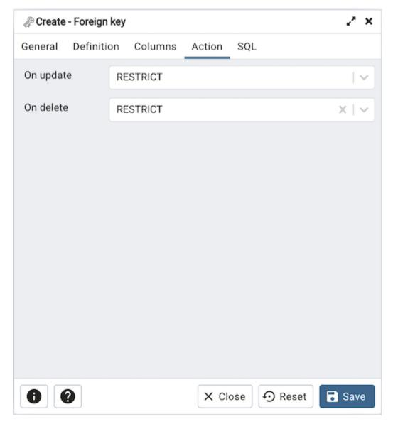
Use the drop-down listboxes on the *Action* tab to specify behavior related to the foreign key constraint that will be performed when data within the table is updated or deleted:
