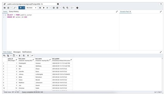
To modify the content of a table, each row in the table must be uniquely identifiable. If the table definition does not include an OID or a primary key, the displayed data is read only. Note that views cannot be edited; updatable views (using rules) are not supported.
