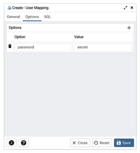
Use the fields in the *Options* tab to specify connection options; the accepted option names and values are specific to the foreign data wrapper associated with the server specified in the user mapping. Click the *Add* button to add an option/value pair.
