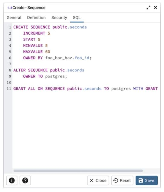
The example shown demonstrates a sequence named *seconds*. The sequence will increase in 5 second increments, and stop when it reaches a maximum value equal of 60.
