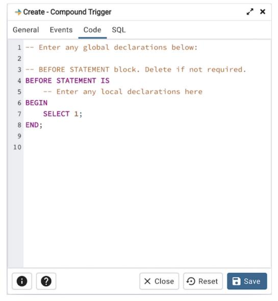
Use the *Code* field to specify the code for the five timing events *BEFORE STATEMENT*, *AFTER STATEMENT*, *BEFORE EACH ROW*, *AFTER EACH ROW*, *INSTEAD OF EACH ROW* that will be invoked when the compound trigger fires. Basic template is provided with place holders.
