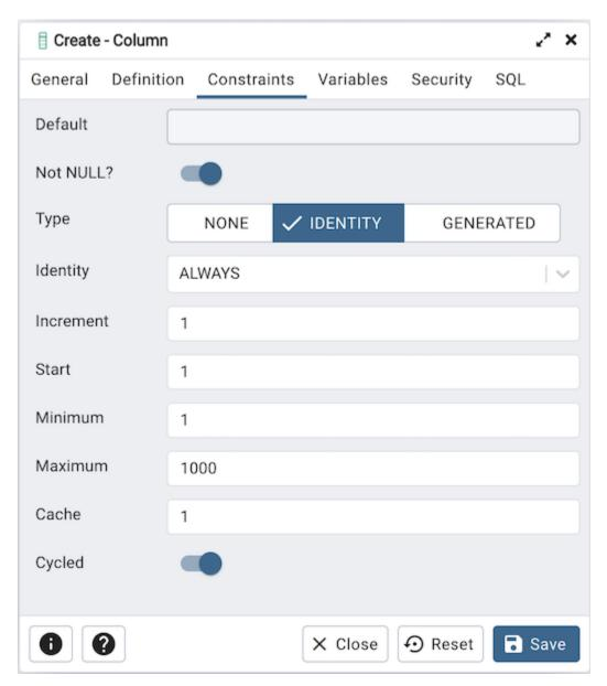
Use the following fields to create *IDENTITY* column. Identity columns are applicable for PG/EPAS version 10 and above.
