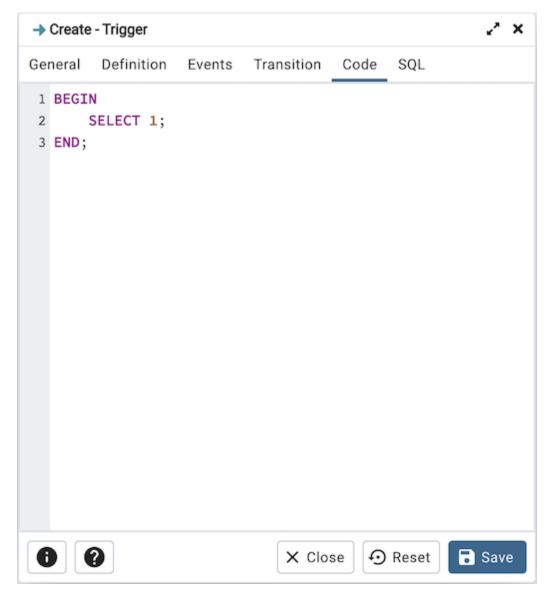
Use the Code field to specify any additional code that will be invoked when the trigger fires.
