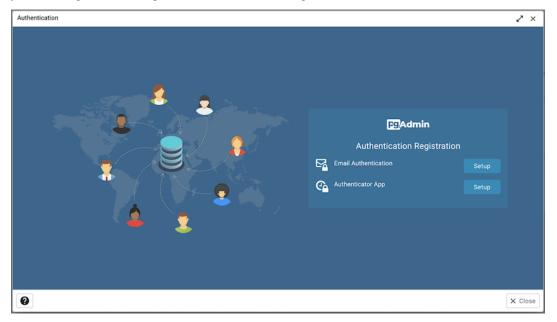
You can also force users to configure the two-factor authentication methods on login by setting *MFA\_FORCE\_REGISTRATION* parameter to *True*.
